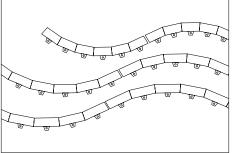
For a concave or convex curve, lay curb units in the same direction.
