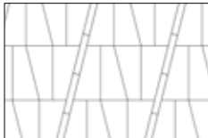
Diagonal 100 x 450 with Boulevard 300 pavers 100 x 450
