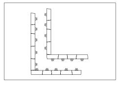
For a 90° corner, simply align curb units at this angle.
