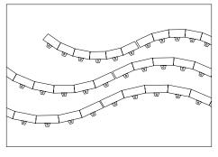
For a concave or convex curve, lay curb units in the same direction.
