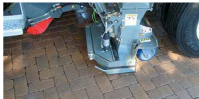
Vacuum truck for restorative maintenance
