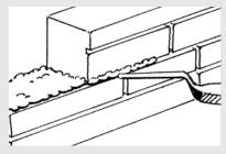
In order to make sure that all the mortar joints have the same colour, tool them when they have the same firmness. It should be noted that the firmer the joints, the darker the colour will be when tooled.
