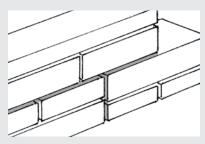
Try to achieve a "mortar joint in. of approximately 6 mm (1/4 in.) thick so that you can obtain an equal appearance throughout the stones.
