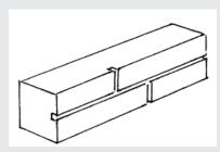
Each stone has different reliefs. This should be taken into consideration when installing the stone.
