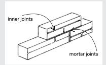
Identify the "mortar joints in. and the "inner joints in.. The basic principle would be to have the "mortar joints in. and "inner joints in. as similar in thickness as possible.
