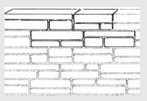
Lamina stone is installed like any other masonry veneer. The units should be installed randomly.
