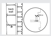
Leave a recessed joint of 6 mm (1/4 in.) deep compared to the deepest stone, so that all joints appear equal.
