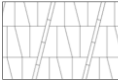
Diagonal 100 x 450 with Boulevard 300 pavers 100 x 450
