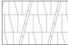
Diagonal 100 x 450 with Boulevard 300 pavers 100 x 450
