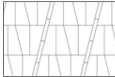
Diagonal 100 x 450 with Boulevard 300 pavers 100 x 450
