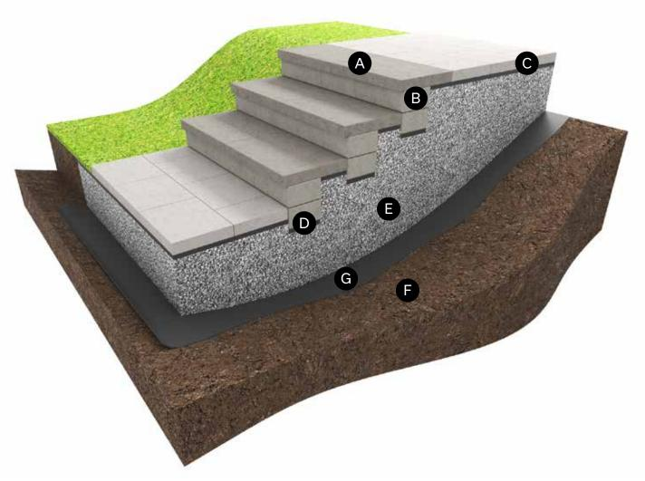
All step and riser units must be bonded together with Techniseal concrete adhesive.
